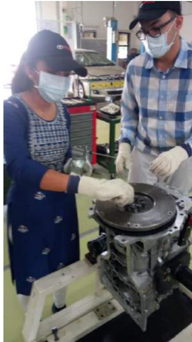
Mr. Kiran Kumar, Trainer given hands on experience of Dismantling and Assembly of Gasoline Engine by participants
