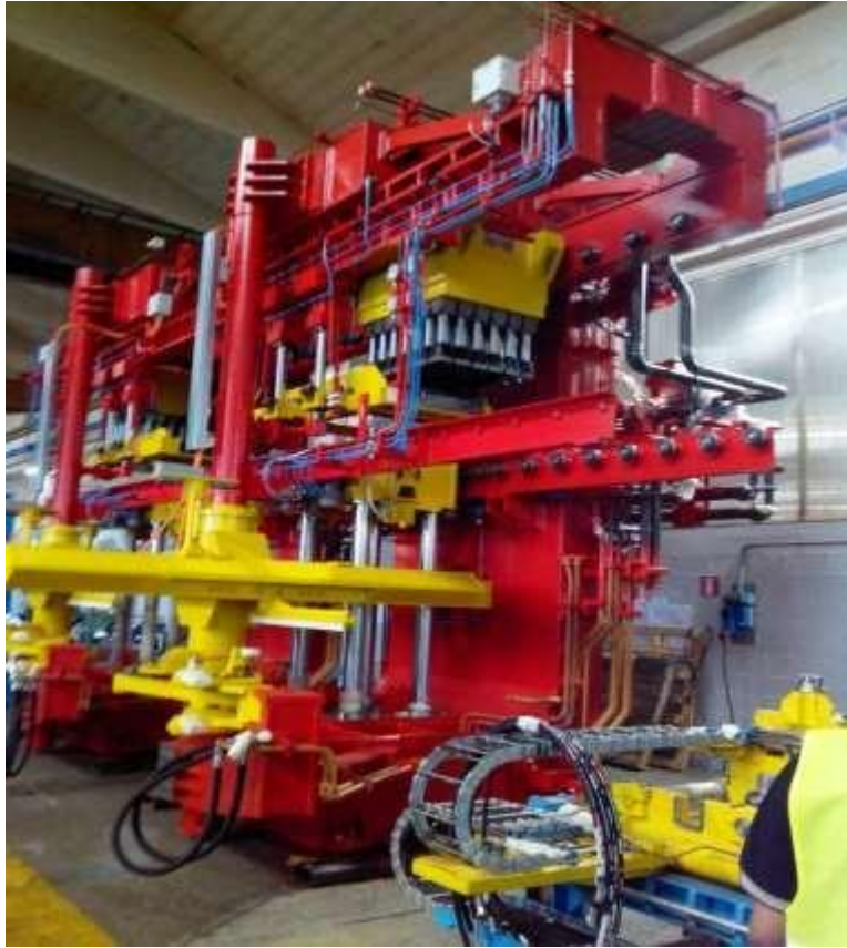
Fig: High pressure moulding machine –savelli italy, Lamina Foundries Ltd. Nitte
