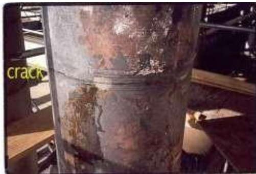
Main steam pipe weld failure
