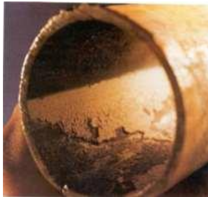
Oxide layer formation in the boiler tube
