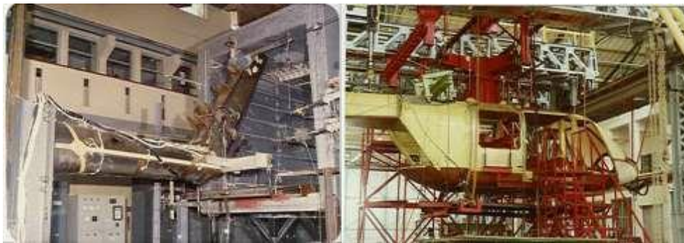
Fig 1: Experimental setup for Static Strength & Fatigue Tests on Components (Sub-assemblies & Full Airframe) located at RWRD Centre, HAL Bangalore
