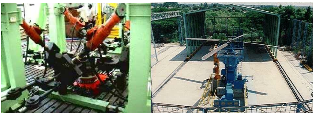
Fig 2: Main rotor hub test and Main rotor whirl tower
