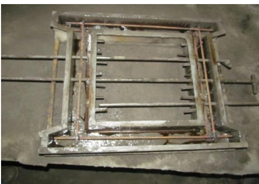
STEP 2: The iron rods are inserted inside the iron mould to provide grip for the concrete mould.
