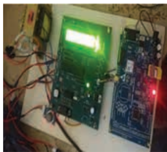
Fig.4: shows the implementation of proposed device to monitor air quality
